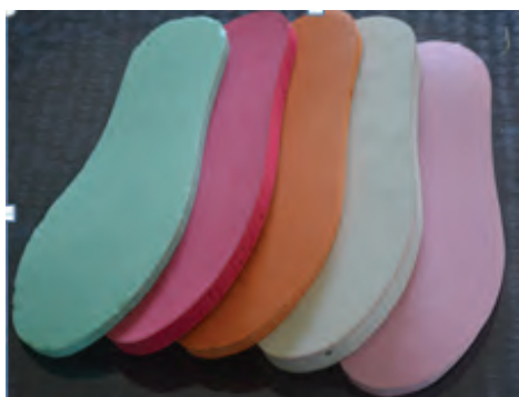
Figure 2. Orthotic insoles produced from 100 % natural rubber
