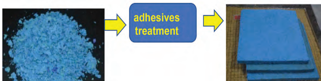
Figure 5. Flow chart for the production tiles from glove powder
