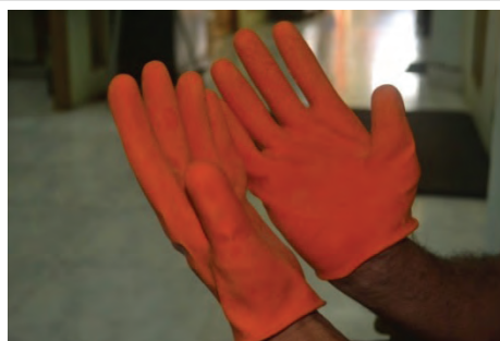
Figure 4. Hand gloves produced from room temperature vulcanization.
